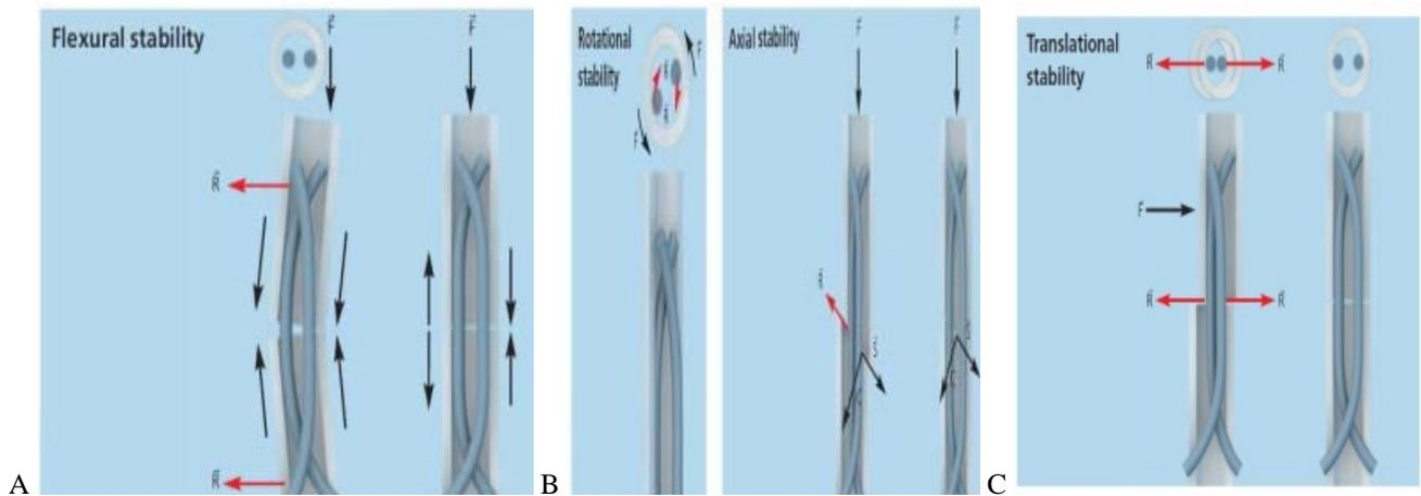
**Figure (2):** stability of (E.I.N)<sup>(9)</sup>. A: the flexural stability of (E.I.N) B: the rotational and axial stability of (E.I.N) C: the translational stability of (E.I.N)
