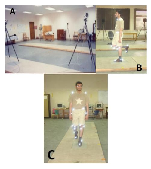
Fig.6: a-Motion capture unit. B &C- Force plate unit and reflective markers
