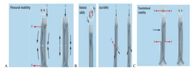
**Figure (2):** stability of (E.I.N)<sup>(9)</sup>. A: the flexural stability of (E.I.N) B: the rotational and axial stability of (E.I.N) C: the translational stability of (E.I.N)
